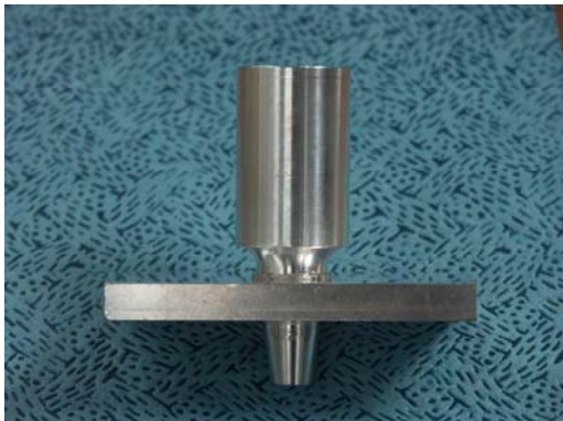
Figure 2.21: Picture of a similar FTP weld using AZ91D-T6 as base material [126] .
